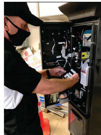
Parking Enforcement Officer Jason Jerard converting a direct powered meter from the parking garage to a solar powered on-street version.
