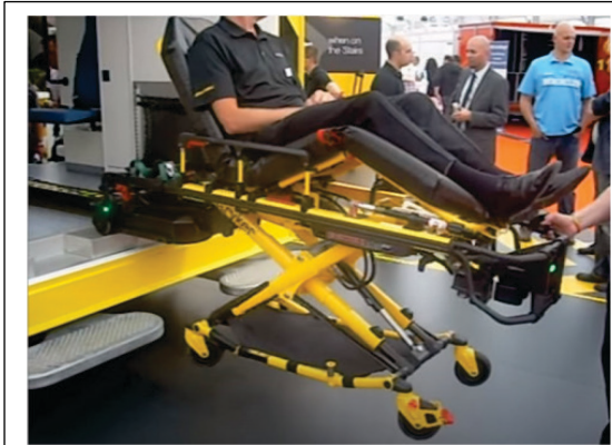
Demonstration of the Power Load System
