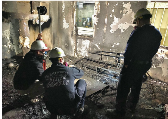
Post fire examination of a burn cell and the effect of ventilation on fire patterns.
