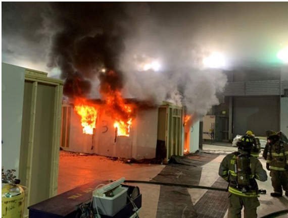
A burn cell under fire conditions after the windows failed due to the intense heat.
