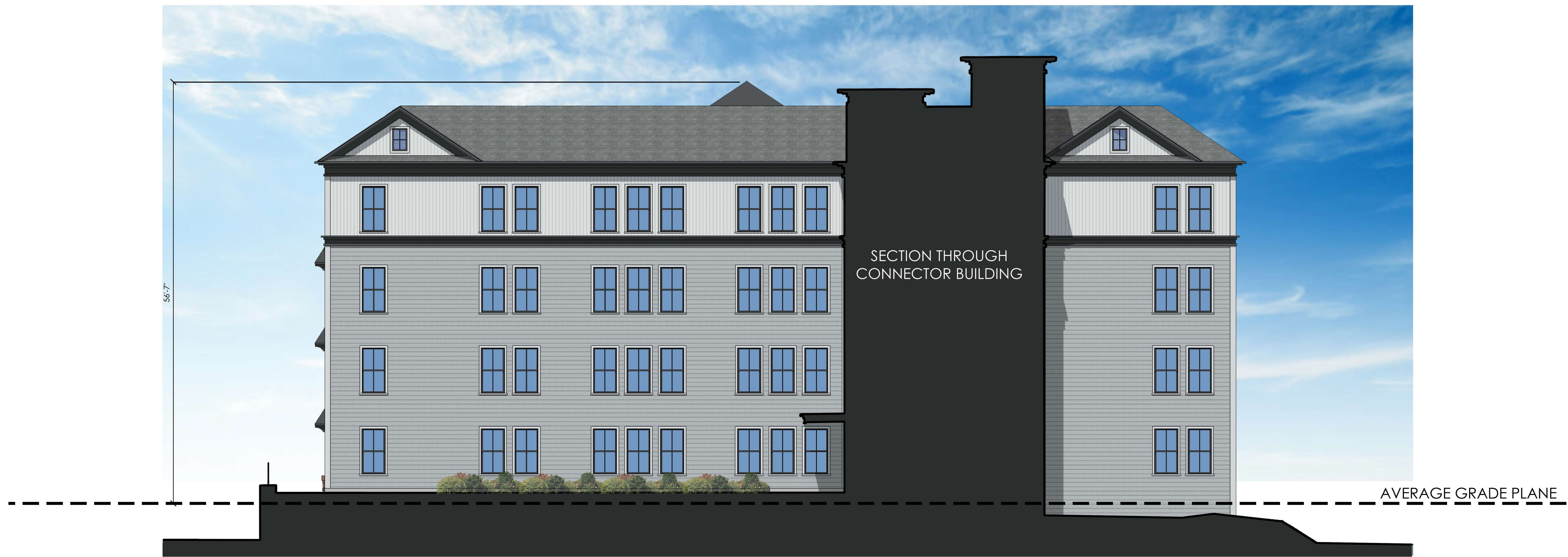
2 NORTH ELEVATION AT NEW ADDITION (COURTYARD) 1/8" = 1'-0"
