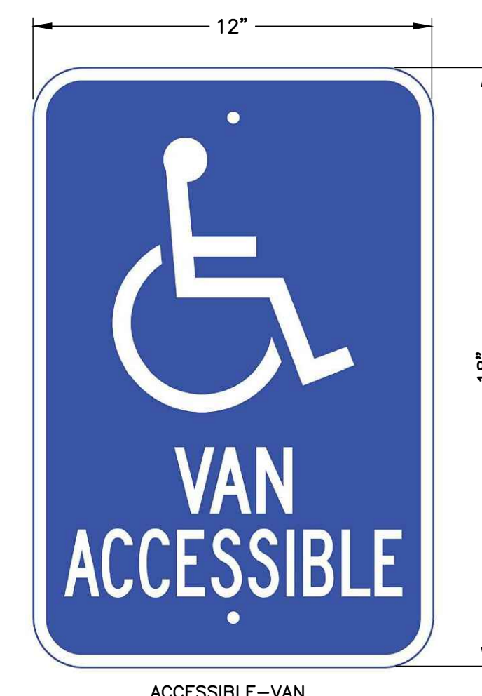
ACCESSIBLE SIGNAGE DETAIL
