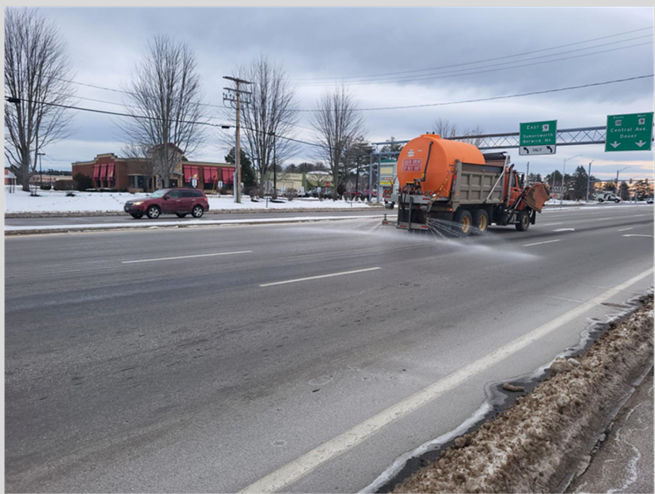
One of Dover's brine applicators applying a brine at a rate of 50 gallons per lane mile with penetrative nozzles before a storm.
