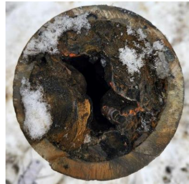
1880s vintage 4-inch cast iron water main within Angle Street that is being replaced due to repeated failures. The pipe's capacity has been reduced significantly due to build up within the pipe.
