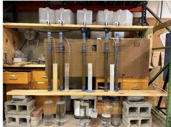
Picture of the constant head infiltration rate test being conducted at UNH in conjunction with the City of Dover Engineering Department.
