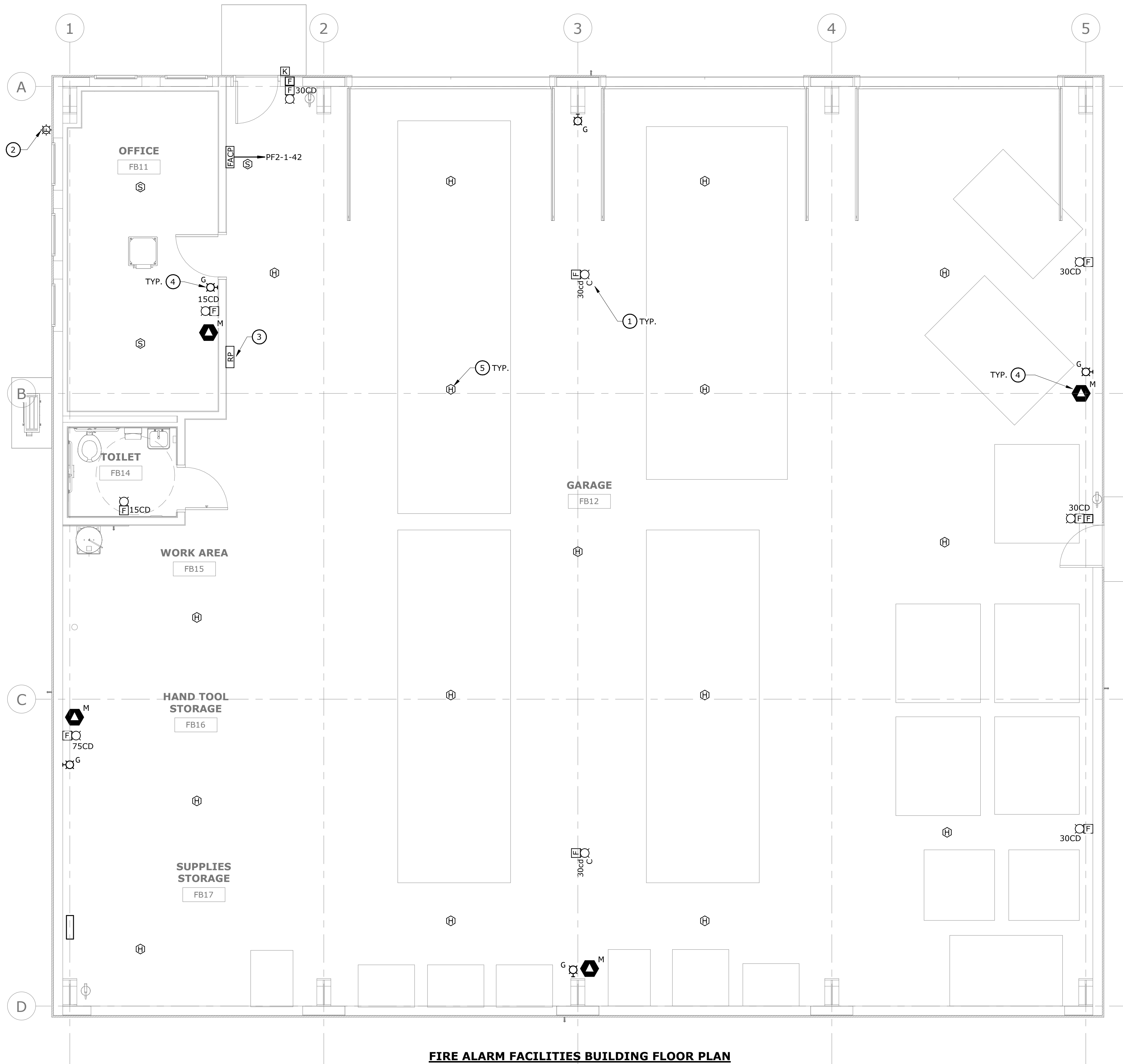
FIRE ALARM FACILITIES BUILDING FLOOR PLAN SCALE: 1/4" = 1'-0"
