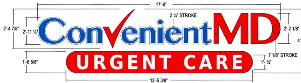
OPTION 1 ITEM B - (1) SET LED CHANNEL LETTERS SCALE: 3/8"=1'-0"
