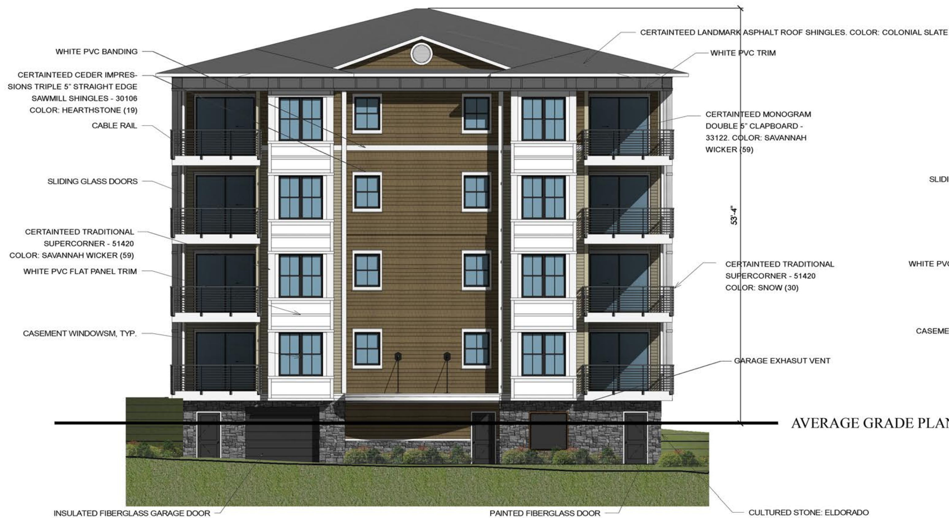
① BUILDING 4 SOUTH ELEVATION 1/8" = 1'-0"
