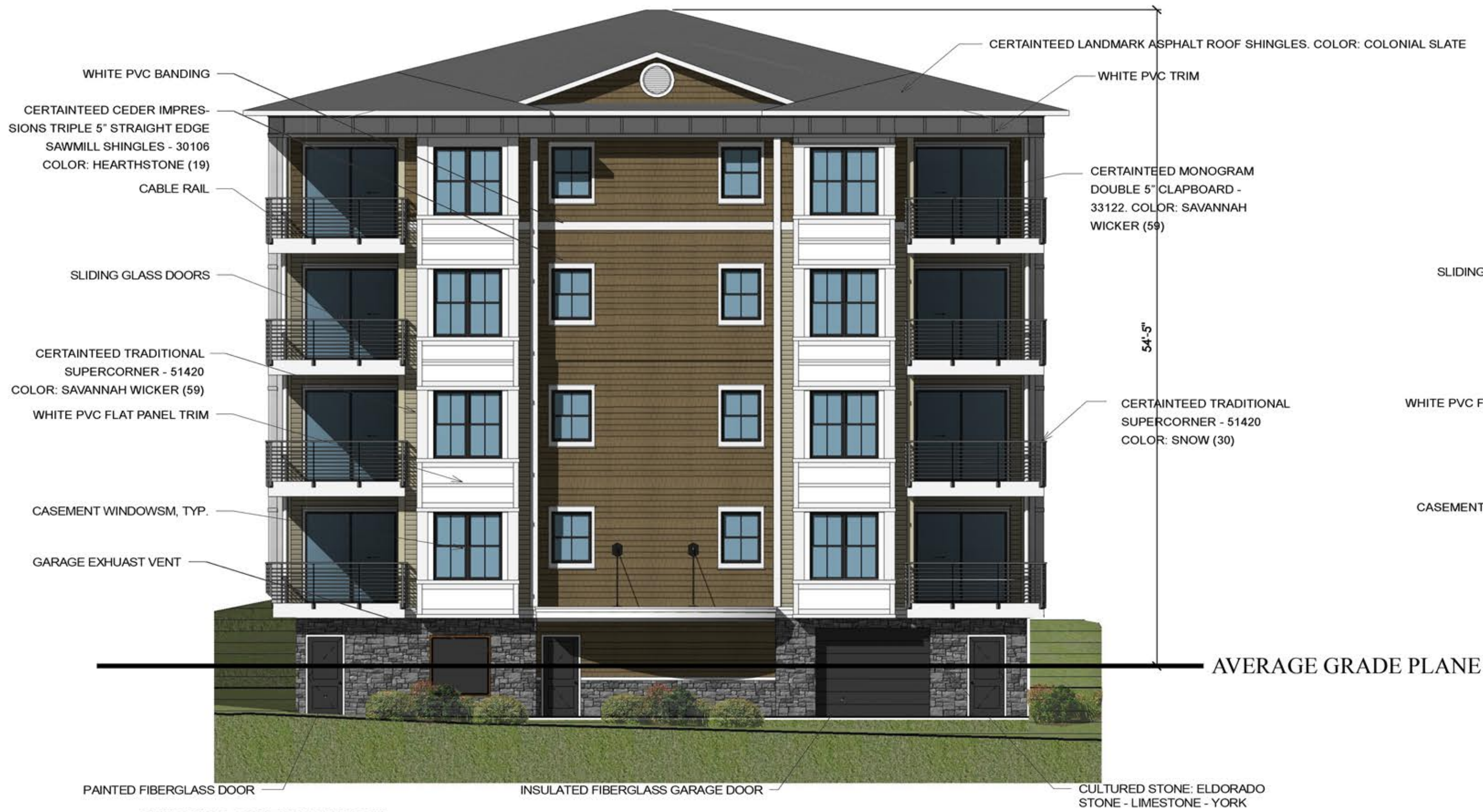
① BUILDING 2 SOUTH ELEVATION 1/8" = 1'-0"
