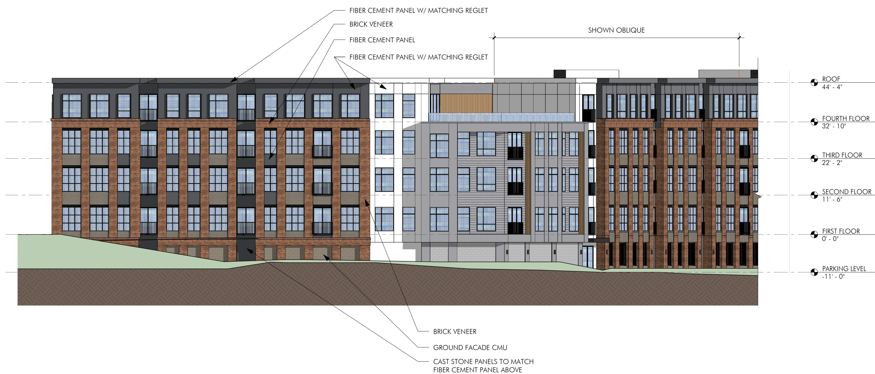
3 NORTH ELEVATION - RIVER STREET ADJACENT PUMP HOUSE 1/16" = 1'-0"
